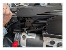
For 17.25in seat height only: Reinstall the original seating assembly bolts, replacing the lower washers with the provided MIL-Spec 5/16 ID washers. Torque to 25 ft-lbs.
