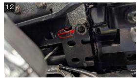
Check that the bracket is level (Figure 15) and then tighten the bolts in the following order: the rearmost rear bolt first, then the front top bolt, then the forwardmost rear, then the front lower bolt. Repeat steps 2 and 3 on the other side. Then, reinstall the front battery cover (Figure 16).
