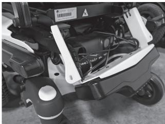
A Caution: Make sure the Rear SmartFrame is rotated out of the way and watch for interference as you flip the seat open, to avoid damaging the SmartFrame. It may be necessary to remove the plastic caps on the rear pivot bolts with a small flat head screwdriver. Alternatively, use a kickstand to hold the chair open enough to access the batteries but closed enough to prevent damaging the LUCI SmartFrame.
