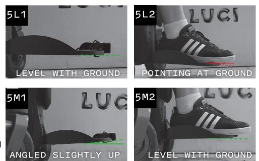
• Note: If the driver typically drives with the footplate raised, the Scout should be adjusted, following the instructions in Step 5B.
