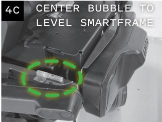
Make sure the bubble is between the lines on the level taped to the SmartFrame and tighten all four screws (Figure 4C). The manufacturer recommends 13.6 - 14.9 N-m (120 - 130 in-lb) of torque on these fasteners. Remove the bubble level once the SmartFrame is level and secure.
