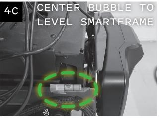
Make sure the bubble is between the lines on the level taped to the SmartFrame and tighten all four screws (Figure 4C).
