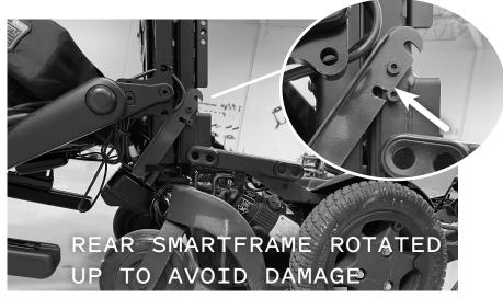
3. Close the seating assembly and reinsert the thumbscrews. Loosen the Rear SmartFrame bolts, adjust the SmartFrame so the top edge of the bracket is level with the ground, and tighten all four bolts. The manufacturer recommends 13.6 - 14.9 N-m (120 - 130 in-lb) of torque on these fasteners. Ensure all cables are neatly routed to avoid pinching or dragging.
