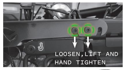
2. Remove the two thumbscrews that keep the seating assembly down. Flip the seating assembly back and swap the batteries as you normally would.
