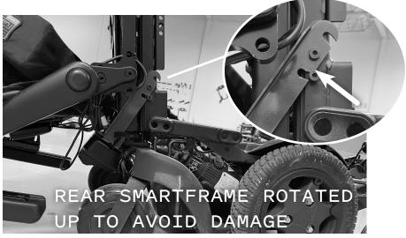
3. Close the seating assembly and reinsert the thumbscrews. Loosen the Rear SmartFrame bolts, adjust the SmartFrame so the top edge of the bracket is level with the ground, and tighten all four bolts. The manufacturer recommends 13.6 - 14.9 N-m (120 - 130 in-lb) of torque on these fasteners. Ensure all cables are neatly routed to avoid pinching or dragging.
